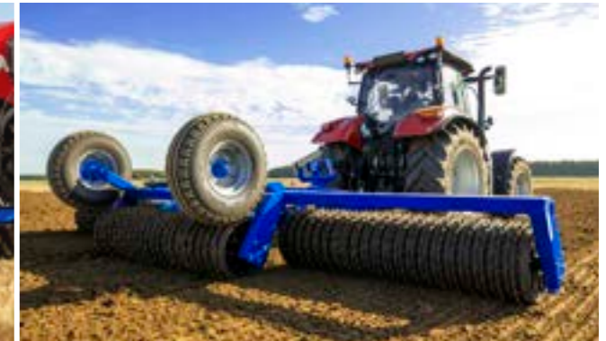
4. The machine is put in the float position and is now ready for use.
