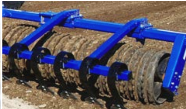
Mounted with hydraulically adjustable cracker board.
