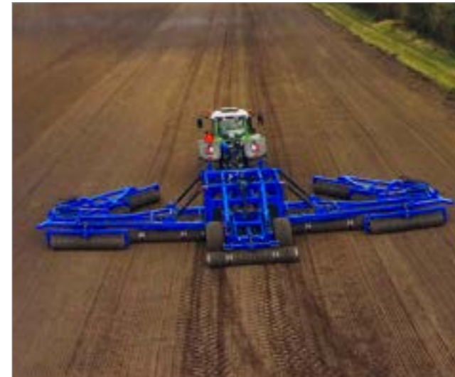
3. Once the roller sections are lowered to the ground, the outer side sections are rolled out to the working position.
