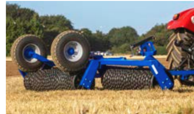
3. The roller sections are lowered to the working position and the wheels are automatically raised.
